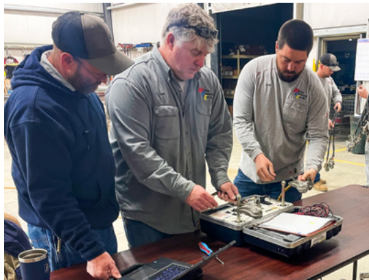
ABOVE: Our Olmitz crew inspects and measures the length of each ground chain before testing.
