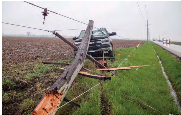
The danger of an accident can be increased greatly when it involves power poles and line. Remember, unless you are otherwise endangered, stay in the vehicle and call 911 and ask the dispatcher to notify the utility.
